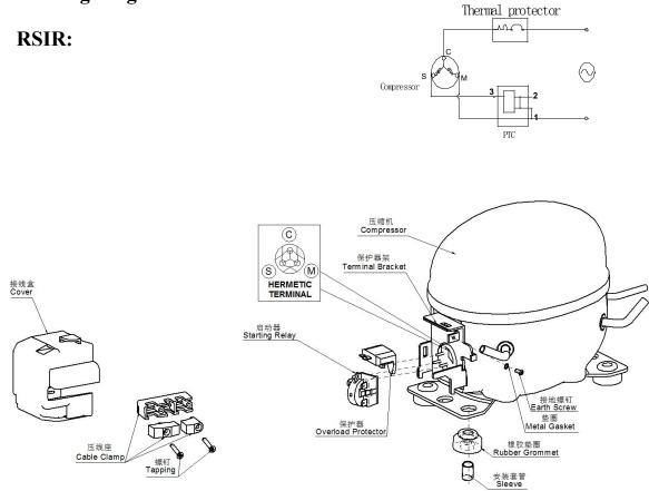
Note: Each of the starting relay, the thermal protector, the spring tap, the terminal cover and the screw assembly is separately provided by our company.
